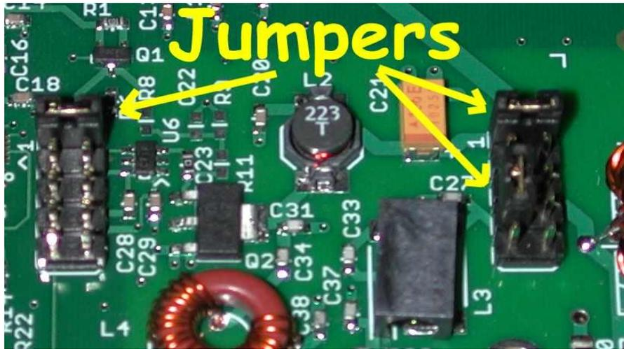
On P4, pins 1 and 2 need a jumper. (Input clock)
