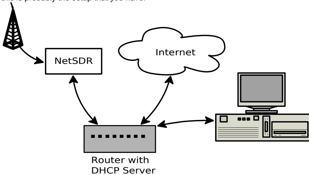
With this configuration, the default settings of the NetSDR and SDR-IP will automatically be discovered on the network and be assigned an IP address. Spectravue should be able to find and connect to it without any further configuration.
