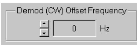
This edit box provides a way to offset the filter and display frequency for receiving CW tones. This is essentially the tone frequency that will be heard in the CW mode when the display frequency is exactly the same as the incoming signal.
