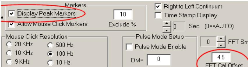
In the direct input mode of the SDR-14, a value of 4.5dB will be very close since this is the level in dBm where the A/D begins to clip. If the internal preamp or an external one is used, then one must change the value accordingly.
