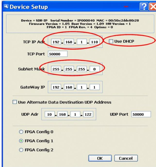
Make sure the “Use DHCP” is not checked and then enter you desired manual IP address and subnet mask values.
