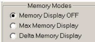
Three radio buttons are used to select the memory modes.
