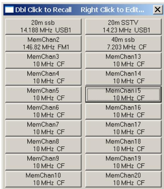
Memory channels are setup by first setting up SpectraVue's center frequencies and both demodulation channels to the desired settings. Then right click on the desired memory channel button to bring up the individual setup menu. Click on the "Clone Current Setting" button to load the memory channel with the current SpectraVue settings. One can also edit the channel text name that will be displayed on the memory channel button.
