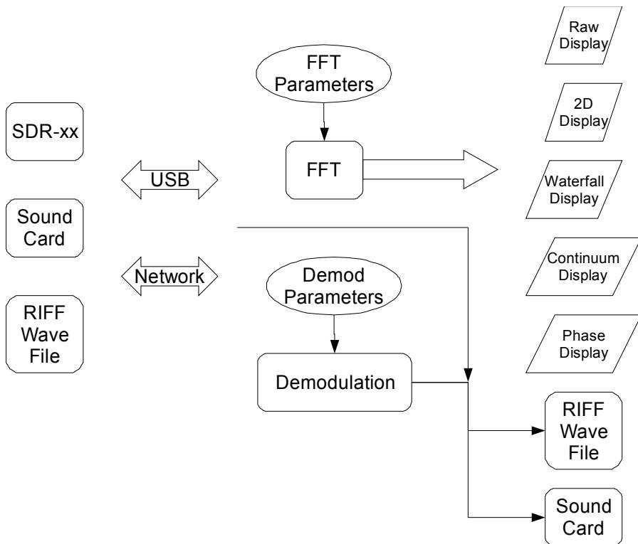
SpectraVue takes as input sources a variety of SDR-xx Software Defined Receivers from RFSPACE Inc, A PC Sound Card, or RIFF .wav file. The FFT (Fast Fourier Transform) is a math transform that converts the time domain data
