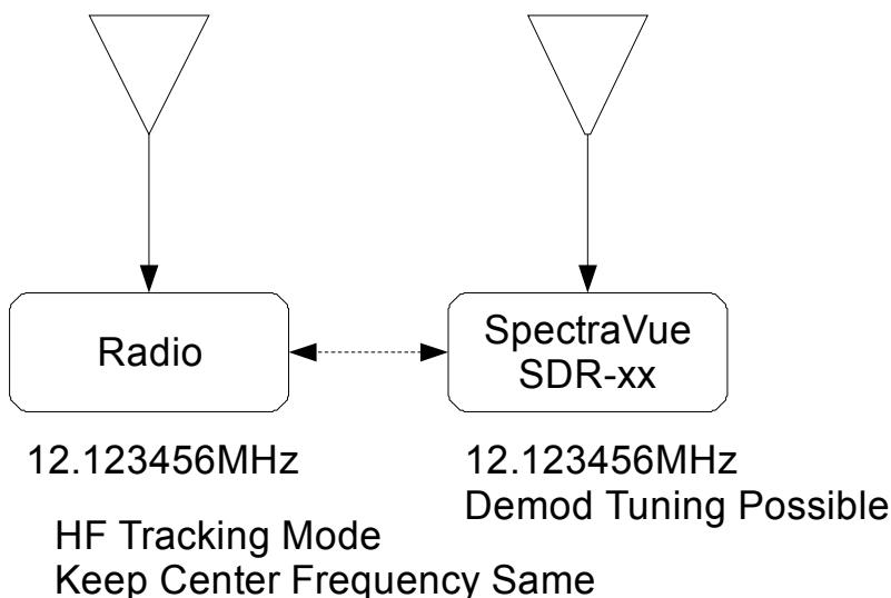
HF Tracking, Allow independent tuning within HF band
