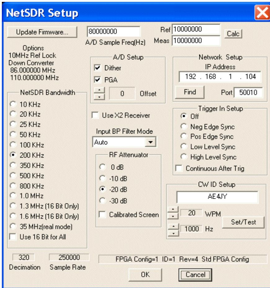
This setup menu is used to set the main parameters of the NetSDR hardware.
