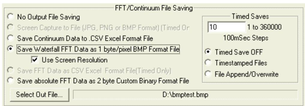
This menu specifies a 1 byte per pixel .BMP graphics file of the waterfall display to be written. If the "Use Screen Resolution" box is checked, the image width will be the same as the screen pixel width. This mode creates images that are the same size as the program screen for easy viewing and reduced file size.
