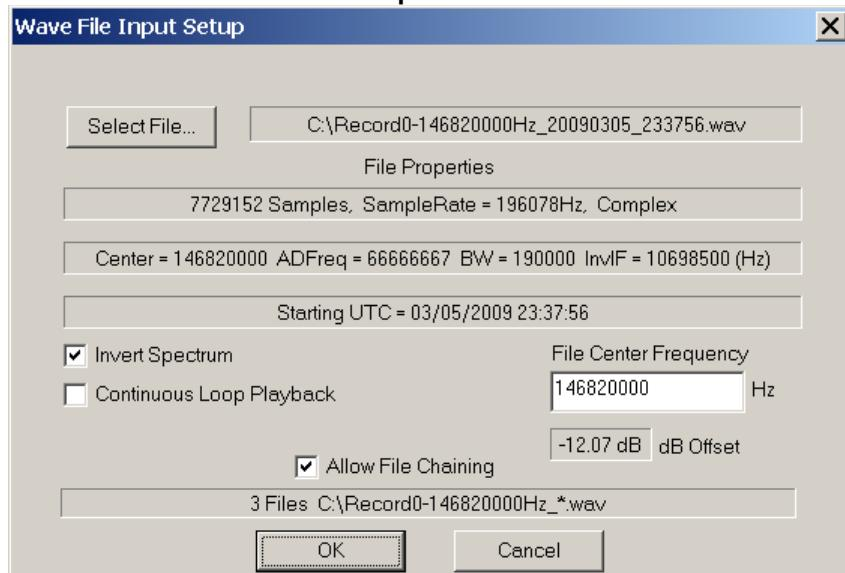
The Wave file input menu allows the user to specify the wave file path and also whether to invert the spectrum or play the file back in a continuous loop.
