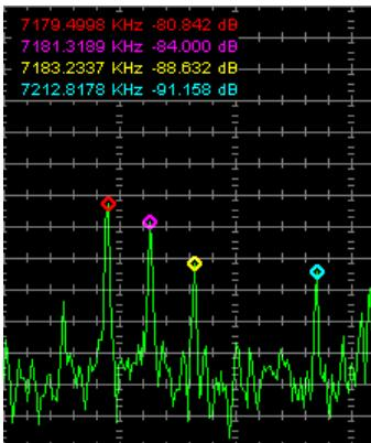
This is a more accurate way of obtaining frequency and amplitude since the actual FFT value is used and not the screen accuracy
