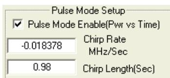
This check box changes the operation of Spectravue from frequency domain display to time domain display. This mode is a special mode for applications where power versus time is more useful than power versus frequency.
