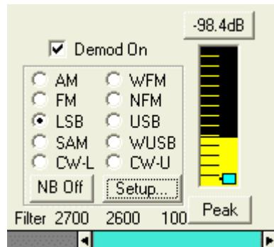
The “Demod On” check box enables or disables the demodulator section. It is only available when the SDR-xx bandwidth is within certain ranges.
