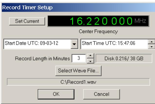
The automatic timed record setup requires the user to select the center frequency, the starting date and time in UTC as well as the run time in minutes and base file name.
