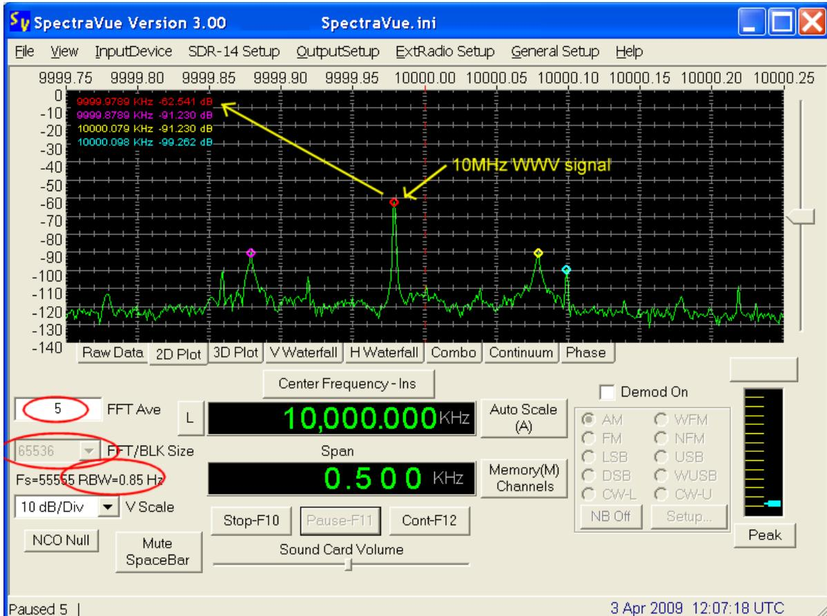
4. Stop or pause the capturing and open the SDR-xx Setup menu. Notice the measured frequency has been automatically placed in the box(if you had peak markers checked and it was marking the correct reference peak) One can manually enter the Reference and Meas frequencies if not using a 10MHz reference.
