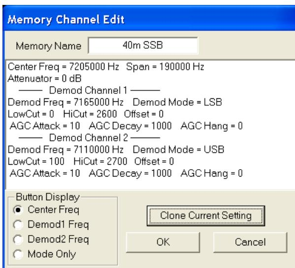
The Button Display group of selections allows the user to pick what type of frequency is displayed on the memory button. The Center Frequency(CF) or one of the demodulation channel frequencies. If demodulation frequency is chosen then the demodulation mode followed by a 1 or 2 denoting which demodulation channel is displayed after the frequency.
