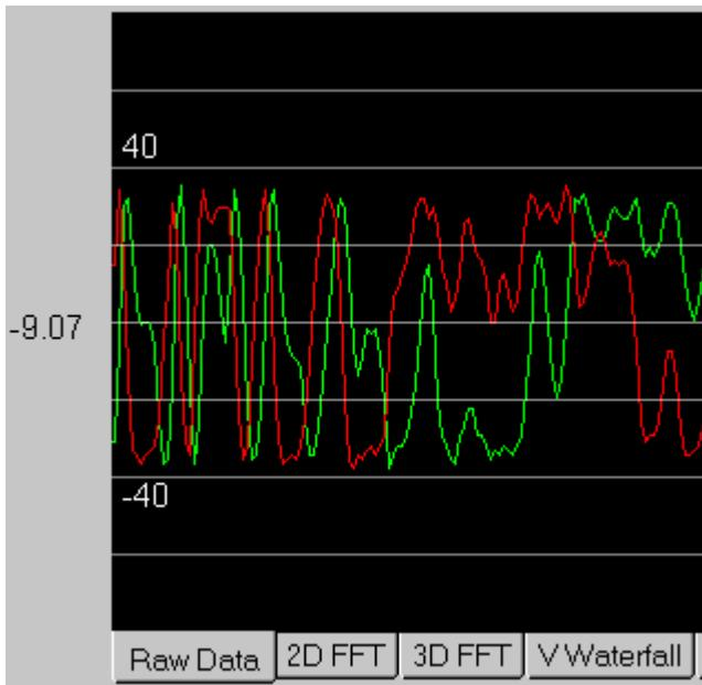
If it is real data then there is only one trace. Complex data is displayed as two different traces with different colors. The two numbers in the display area are the max and min values of the incoming signal. The range of inputs is a 16-bit value or 0 to +/- 32767.
