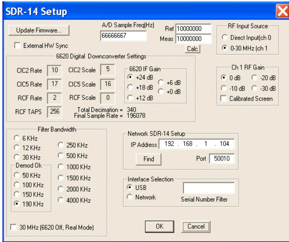
The A/D Sample Frequency can be entered here. Nominally it is 66,666,667Hz but this number can be changed to the actual oscillator frequency if more accurate frequency measurements are desired.
