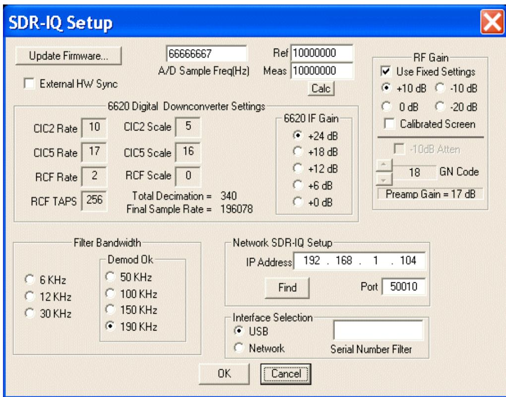
This setup menu is used to set the main parameters of the SDR-IQ hardware.
