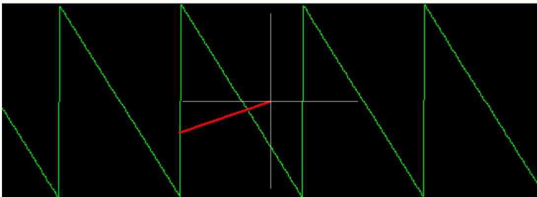
The Continuum range is +/- 180 Degrees where zero is at the center of the screen and +180 at the top.
