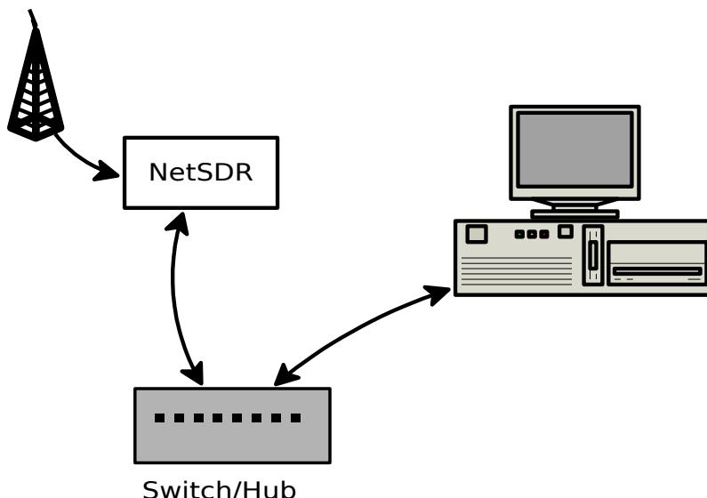
There are two items you need to set in order to get the radio and PC to talk to one another. One is the IP address and the other is what is called a Subnet mask. The Subnet mask is just a filter value that only allows network addresses
