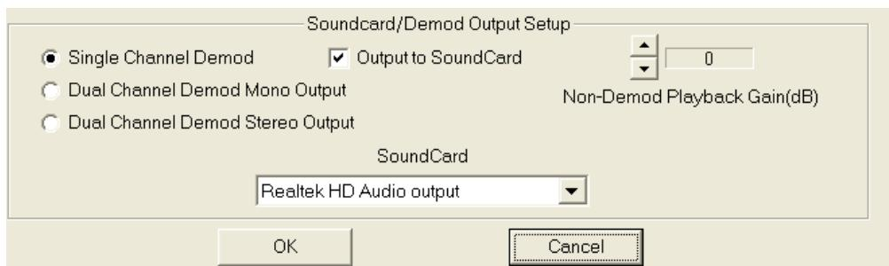
The Soundcard output menu allows enabling the soundcard for output. This is primarily for listening to demodulated signals but can also be used in playing back wave files or listening directly to I/Q data if the soundcard supports the input sample rate.
