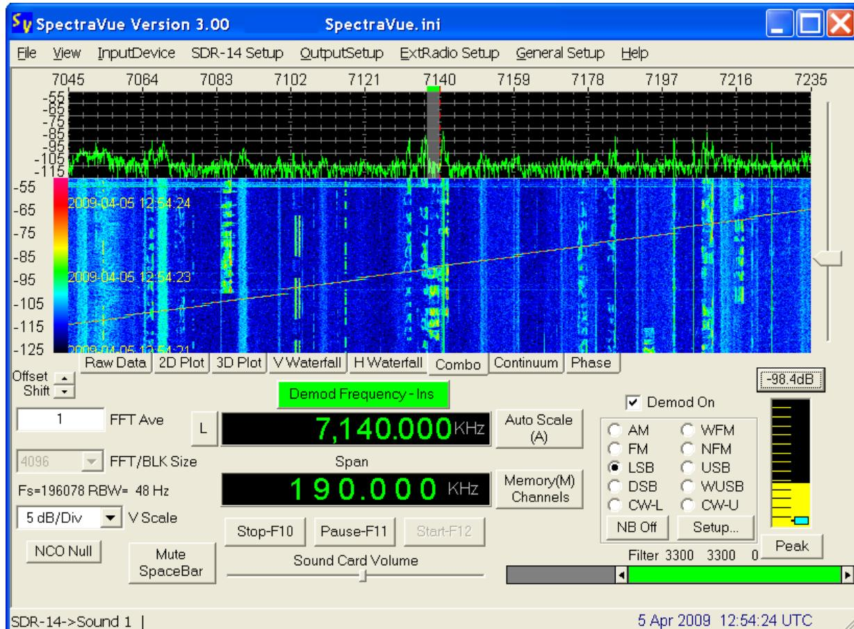
The Main Screen should look similar to this when first run. The receive center frequency can be changed by clicking in the main display area, using the mouse scroll wheel, or entering the frequency digits directly into the frequency control.
