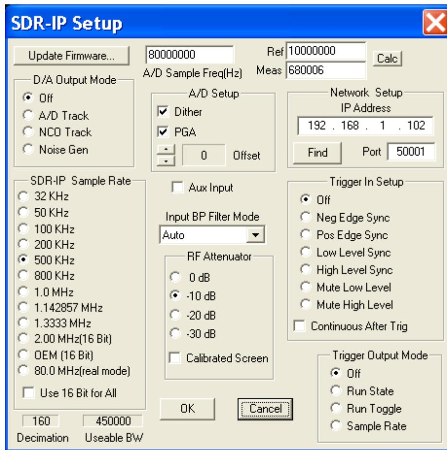
This setup menu is used to set the main parameters of the SDR-IP hardware.
