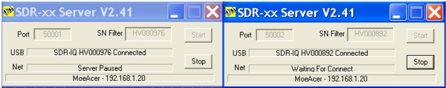
Press Start to turn on each of the servers. In SpectraVue, using the Find button should display all the radios in a list and you can pick the desired one. The same trick to have multiple instances of Spectravue by creating multiple copies of the Spectravue.exe file can be used to run several instances on the same PC where each one is talking to a different radio. (See Hints and Tricks section 7)
