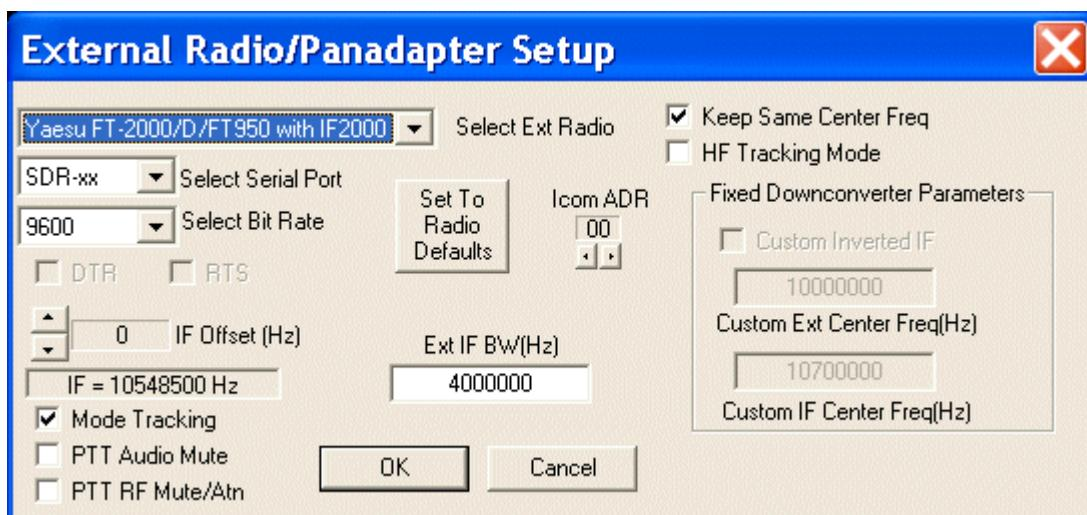
Several radios are directly supported that allow communication between SpectraVue and the radios that the frequency settings track each other. Normally the radio has an IF output that is fed into the SDR-xx and is automatically set up as to frequency and whether it's spectrum is inverted or not.
