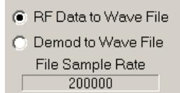
These two buttons select whether the raw RF data samples are saved to the .wav file or if the demodulated audio samples are saved to the file. The file sample rate is shown in the text box.
