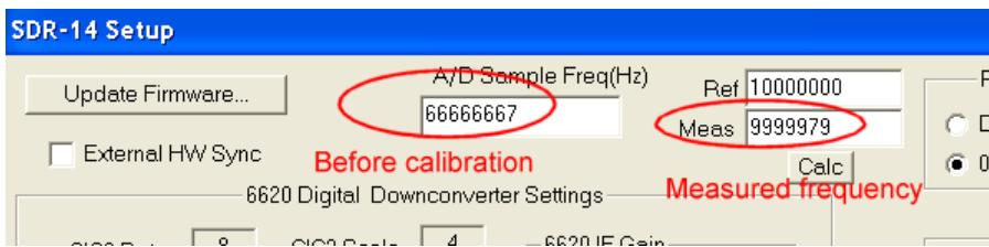
5. Click on the "Calc" button and the new A/D Sample Frequency is calculated. The "Meas" box will revert to the Ref frequency so one doesn't accidentally keep scaling the A/D sample frequency.
