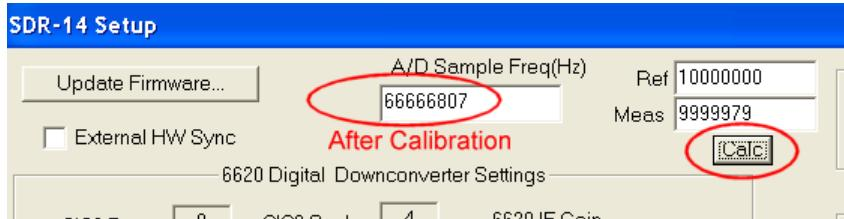
6. Go back to the main screen and start the captures again to verify that the new calibration has taken affect. One may have to perform this a few times to iterate the error to zero if the signal is noisy or the SDR-xx is still warming up.
