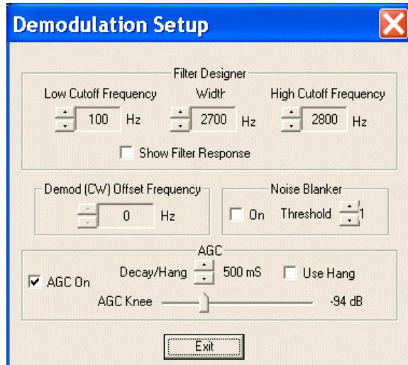
AGC can be turned off and then the slider controls the signal gain. Be careful with this as a strong signal will overdrive the soundcard and cause quite a racket.
