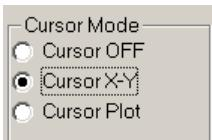
The X-Y mode shows the frequency and amplitude of the cursor mouse position on the screen.
