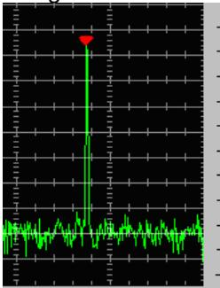
2. Left click on another part of the waveform and the first red marker freezes at the last value of the spectrum and a new yellow marker attaches to the new FFT position. It can also be moved with the function keys. The numeric value of the delta between the two markers is now shown in the upper left of the 2D display screen.
