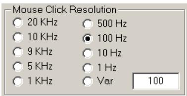
This group of menu items allows the selection of how to round off the frequency when using the mouse to click close to a signal on the display.
