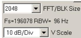
Basic information of the current FFT settings are shown on the lower left side of the main screen. Fs is the current sample frequency and RBW is the FFT resolution bandwidth(ie the smallest frequency resolution of the FFT display).
