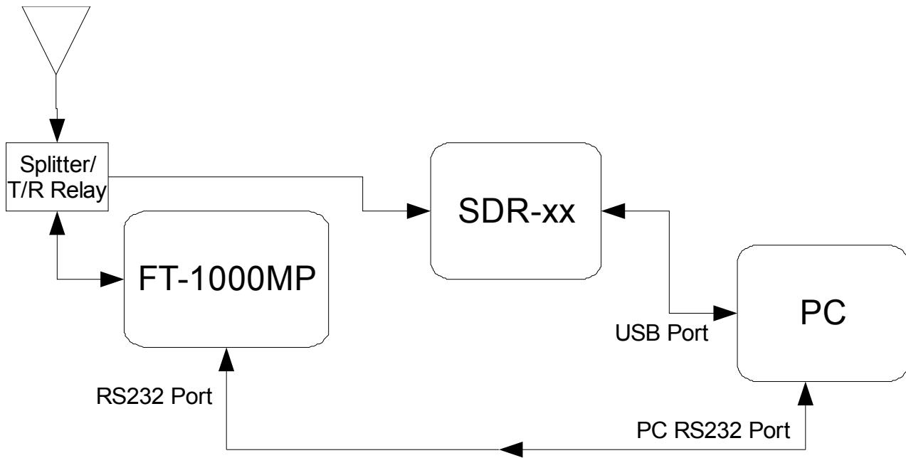
**User must also add some sort of signal splitter and/or T/R relay when using the transceiver so as not to transmit RF power into the SDR-xx.**
