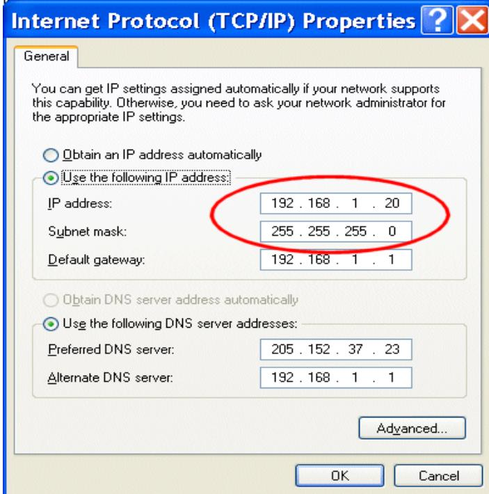
Make sure the "Use the following IP address" is selected and then enter your desired IP address, and subnet mask values. If you are not connecting to other networks like the Internet, you can leave the Default Gateway blank. The DNS server again is used for Internet connectivity and is not needed just to connect to the radio.
