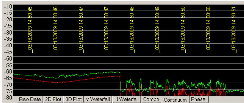
FFT amplitude power is in dB referenced to full scale (a single sine wave with an amplitude of +/-32767 or 16 bits). This can be calibrated to say dBm by entering a dB offset in the FFT Setup menu.
