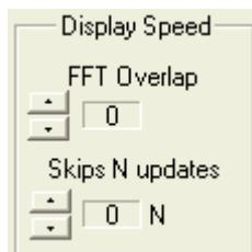
The "Skip N Updates" mode forces the program to skip display updates in order to reduce computational load on the processor. As the number of N grows larger, the more updates that are skipped by the display. A value of zero runs the display at full speed.
