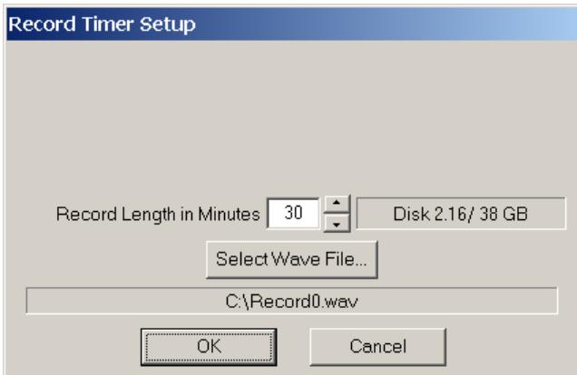
The manual record mode only sets the file root name and the maximum recording time. The disk space requirements are estimated based on the time limit and current file sample rate.
