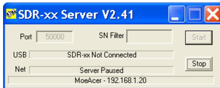
Connect the SDR-xx USB cable to the remote PC and apply power to the SDR-xx if required. The server should connect to the SDR-xx and the following status should result.
