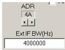
The Ext IF BW edit box allows the user to specify what the useable bandwidth of the radio IF. This can be used to limit the IF to regions that are more flat or that do not contain as many spurious signals.
