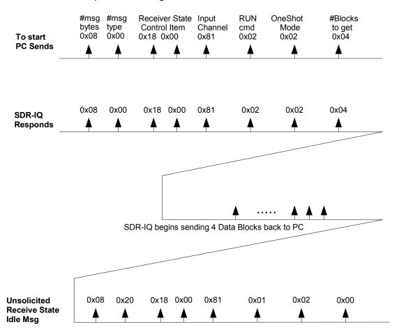
Target sends unsolicited Receive state idle message after last data block
