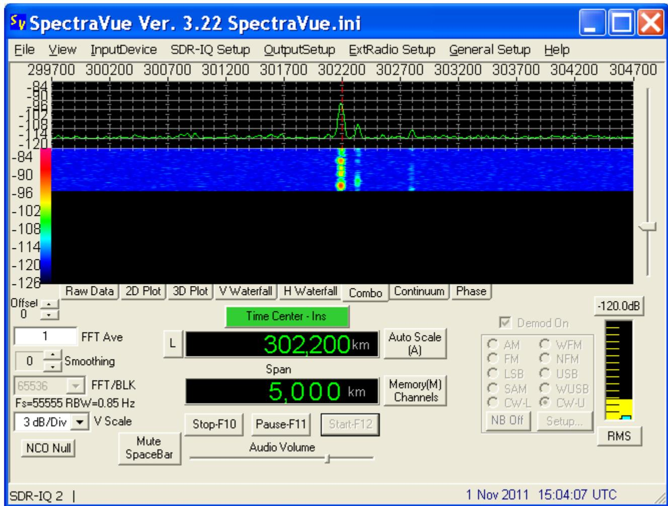
There are multiple pulses due to having several transmitters on the same frequency but shifted in time. Also there are pulse artifacts from the signal since the sweep has blanking intervals that codar uses to be able to listen for reflections while transmitting.
