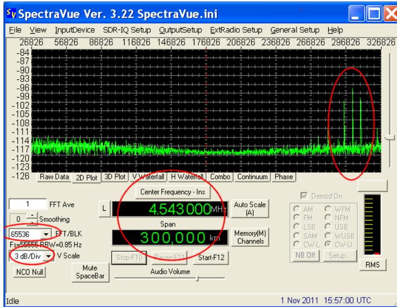
The button above the frequency control toggles the control between center frequency of the radio and the display time(distance) center of the screen. The Span control adjusts the span in time(distance) units. Start out with maximum span to initially find the pulses.
