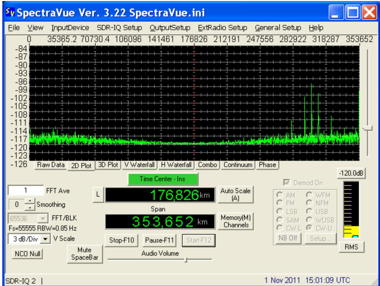
Note the largest pulses position then reduce the span to zoom the screen while readjusting the time center value close to the pulses position until you are able to center it on the screen.
