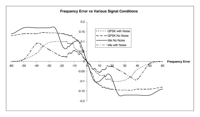
The differential frequency error was originally used to correct the master NCO by itself. Now a secondary phase derived error signal is used once the error gets within 3 Hz. The differential frequency error signal is used when the error signal is large, then the phase derived frequency error kicks in when the error becomes small.
