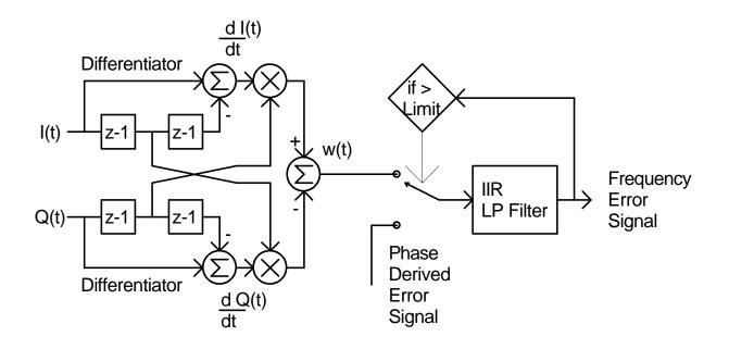
The IIR LP filter are the same type as used in the AGC section with different time constants.
