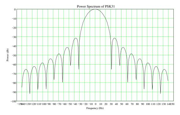
The following FFT scan of a QPSK signal compares favorably with the math model. The vertical divisions are 10 db.
