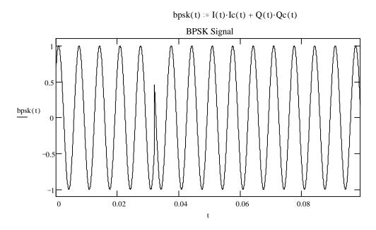
Note the abrupt phase change at time t = .032 seconds. This is not desirable since it makes the PSK signal very wide. One way to limit the bandwidth would be to filter the output signal. PSK31 uses a different method by using waveshaping on the I and Q input signals so that instead of abruptly going from a 1 to a -1, the signal makes a cosine shaped transition between -1 and 1.
