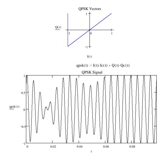
Note that during 90 degree phase changes, the amplitude does not drop all the way to zero as in the 180 degree case.
