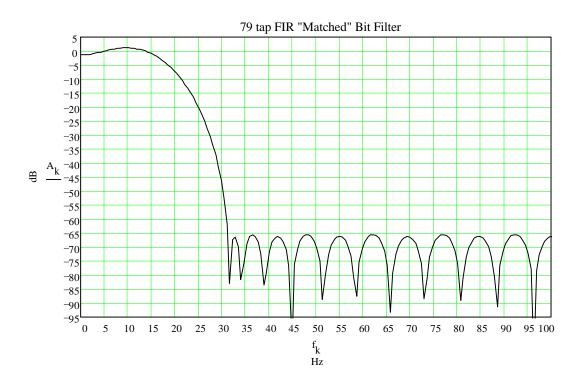
All the FIR filter coefficients were designed using either MathCAD or a program called PC-DSP by DSP Solutions.
