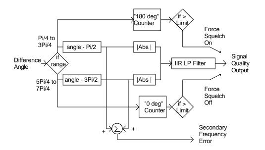
If the incoming difference angle is in the "ZERO" range, the absolute value of the angle and Pi/2 is found. If the incoming difference angle is in the "180 degree" range, then the absolute value of the angle and 3Pi/2 is found. The two values are added together and run through a low pass filter. This is a measure of how far away from the ideal the angle is, and is used for squelch control and signal quality display.
