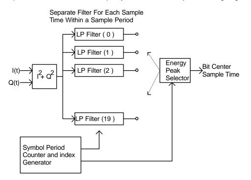
There are about 20 samples per symbol at the 612.5 Hz. Sample rate. The energy in the input signal at each sample time is individually filtered and stored in a filter array. At each symbol period of .032 seconds, the filter that has the most energy is selected and the sample point associated with this sample is assumed to be the center of the data symbol.
