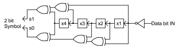
Note that the data bits from the varicode word are inverted before entering the shift register. This is so that the idle stream of all zeros will produce symbols of '10' which are 180 degree phase shifts. This is useful for maintaining symbol sync on the receiver side and being compatible with BPSK.
