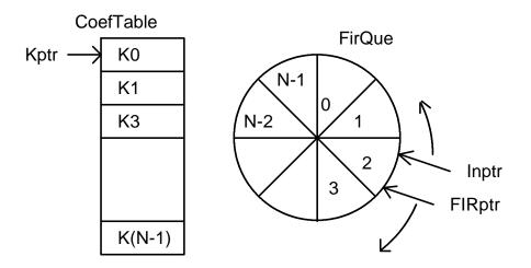
The following code segment shows the general method of implementation. For a decimation type FIR filter, the MAC loop only needs to be performed at the new sample rate. For complex data, the MAC has to be performed on both real and complex parts of the data.
