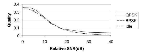
Note how the QPSK signal with very high SNR still has a lower quality signal. This is due to ISI from the bit filter giving the signal some phase jitter.
