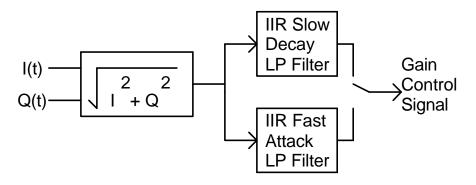
Two different time constants are used depending on whether the signal is increasing in strength or decreasing.
