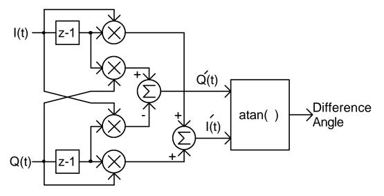
In actuality, a 'C' function atan2(y,x) is used to obtain the angle. It returns a value from -PI to +PI. This still causes some grief if one wants to create a histogram of angles around 0 and around PI(0 and 180deg). If one swaps I and Q, the affect is to map 0 and 180 degrees to +/- 90 degrees. This translates the two ranges of interest( -PI/4 to PI/4 and 3PI/4 to 5PI/4), into the new ranges of PI/4 to 3PI/4, and 5PI/4 to 7PI/4.
