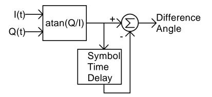
This method has a couple of problems. One is that if I(t) is zero things blow up. Second, there must be extra logic to do the subtraction since the atan function doesn't return a nice 0 to 360 degree range. One must keep track of which quadrant the vectors are in and subtract accordingly.
