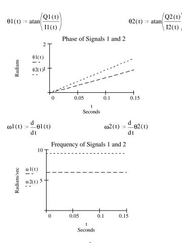
From a dusty calculus book<sup>6</sup> the following identity was obtained that gives the signal frequency as a function of the I and Q signals and their derivatives without the use of the atan() function.
