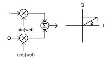
The following MathCad<sup>4</sup> simulation shows how a BPSK signal could be created using the I/Q method.
