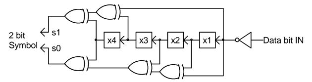
The Viterbi decoder uses the same encoder to try all possible transmitted combinations and calculate an error metric based on how "far away" from each possibility the received symbol is.
