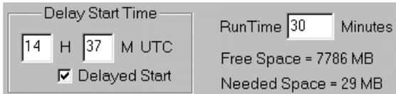
The simulation start can be delayed until a specified UTC time by selecting delayed start, and entering the hour and minute that you wish to start the simulation. This gives up to 24 hours of start delay. The Run Time can be selected from 1 minute to 500 minutes.
